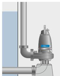
A vertically-mounted, permanent dry well or in-line installation with flange connections for suction and discharge pipe work. Available for 3127, 3153, 3171 and 3202.
