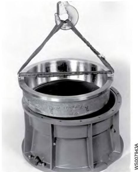
Figure 21: Lifting the wear ring out of the outlet cone
